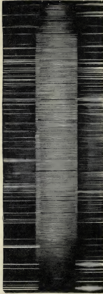
FIG. 187.—Comparison of the Absorption Spectrum of the Sun with the Radiation Spectra of Iron and Calcium, with Common Impurities.
